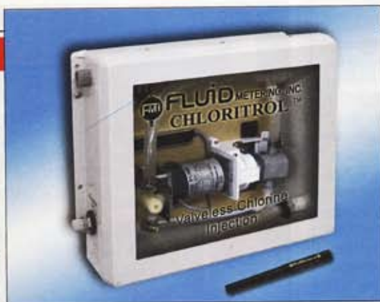
FIGURE 3. Accurately metering liquid sodium hypochlorite presents challenges, but the Chloritrol system's valveless duplex-pump design allows sodium hypochlorite directly into the water main, while a second pump removes out-gas bubbles. Dosage equipment such as this can help processors optimize water treatment programs
